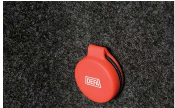
12V Charging Socket can be used to recharge your battery or as a power supply when you need it.
